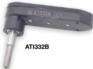
ATI332B Drill Attachment - Flat Head - Gear Drive - Straight Offset. Machined aluminum (hard anodized) housing, recommended drill capacity 1/4", one to one drive ratio, 3 3/16" overall length, 15/16" width, 2 5/16" overall height, 1/2" thick gear drive body, 2 7/16" centerline distance from input shaft to output shaft, 11/32" from centerline of output shaft to end of housing, 1/4" diameter input shaft, #1/4"-28 female threaded output, high speed gear drive with anti-friction roller bearings with (grease) zerk fitting for easy maintenance.
