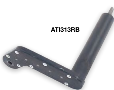
ATI313RB Drill Attachment - Flat Head - Gear Drive - 60 Degree Left Hand Offset. Machined steel housing, recommended drill capacity 1/4", one to one drive ratio, 3 15/16" overall length, 15/16" width, 5 1/16" overall height, 19/64" thick gear drive body, centerline distance from input shaft to output shaft is 3 3/32" by 7/8" of offset, 27/64" from centerline of output shaft to end of housing, 1/4" diameter input shaft, #1/4"-28 female threaded output, high quality gear drive with anti-friction roller bearings.
