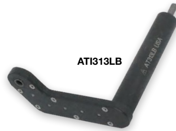
ATI313LB Drill Attachment - Flat Head - Gear Drive - 60 Degree Right Hand Offset. Machined steel housing, recommended drill capacity 1/4", one to one drive ratio, 3 15/16" overall length, 15/16" width, 5 1/16" overall height, 19/64" thick gear drive body, centerline distance from input shaft to output shaft is 3 3/32" by 7/8" of offset, 27/64" from centerline of output shaft to end of housing, 1/4" diameter input shaft, #1/4"-28 female threaded output, high quality gear drive with anti-friction roller bearings.
