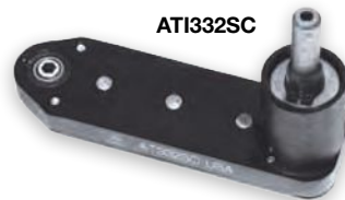
ATI332SC Drill Attachment - Flat Head - Gear Drive - Straight Offset. Machined steel housing, recommended drill capacity 1/4", one to one drive ratio, 3 1/8" overall length, 15/16" width, 2 1/16" overall height, 11/32" thick gear drive body, 2 7/16" centerline distance from input shaft to output shaft, 5/16" from centerline of output shaft to end of housing, 1/4" diameter input shaft, #1/4"-28 female threaded output, high speed gear drive with anti-friction roller bearings. NSN #5130-01-384-6398
