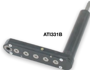
ATI331B Drill Attachment - Flat Head - Gear Drive - Straight Offset. Machined steel housing, recommended drill capacity 3/8", one to one drive ratio, 4 5/32" overall length, 15/16" width, 5 5/8" overall height, 29/64" thick gear drive body, 3 5/16" centerline distance from input shaft to output shaft, 11/32" from centerline of output shaft to end of housing, 1/4" diameter input shaft, #1/4"-28 female threaded output, high speed gear drive with anti-friction roller bearings with (grease) zerk fitting for easy maintenance.
