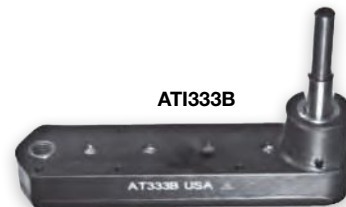
ATI333B Drill Attachment - Flat Head - Gear Drive - Inverted 180 - Degree Straight Offset. Machined aluminum (hard-anodized) housing, recommended drill capacity 1/4", one to one drive ratio, 3 13/16" overall length, 31/32" width, 2 5/16" overall height, 33/64" thick gear drive body, 3 7/64" centerline distance from input shaft to 180-degree rotated output shaft, 21/64" from centerline of output shaft to end of housing, 1/4" diameter input shaft, #1/4"-28 female threaded inverted output, high speed gear drive with anti-friction roller bearings.
