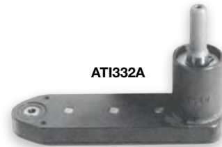
ATI332A Drill Attachment - Flat Head - Gear Drive - Straight Offset. Machined aluminum (hard anodized) housing, recommended drill capacity 1/4", one to one drive ratio, 3 3/16" overall length, 15/16" width, 2 5/16" overall height, 1/2" thick gear drive body, 2 7/16" centerline distance from input shaft to output shaft, 11/32" from centerline of output shaft to end of housing, 1/4" diameter input shaft, #10-32 female threaded output, high speed gear drive with anti-friction roller bearings with (grease) zerk fitting for easy maintenance.
